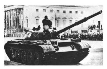
Figure 6-15. T-62 medium tank. The T-62, with a 115-mm smoothbore gun, is replacing the older T-54/55 as the Soviet main battle tank. It can be easily recognized by its five evenly-spaced roadwheels and the bulging fume extractor near the middle of the gun barrel.
